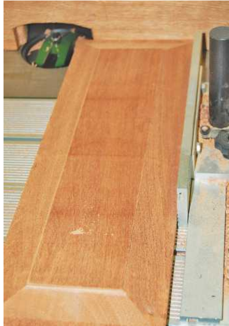
▲ Pic.19 One of the panels, raised & fielded
